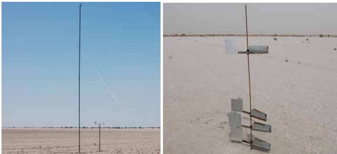
Fig. 12: Wind and erosion measurement stations
