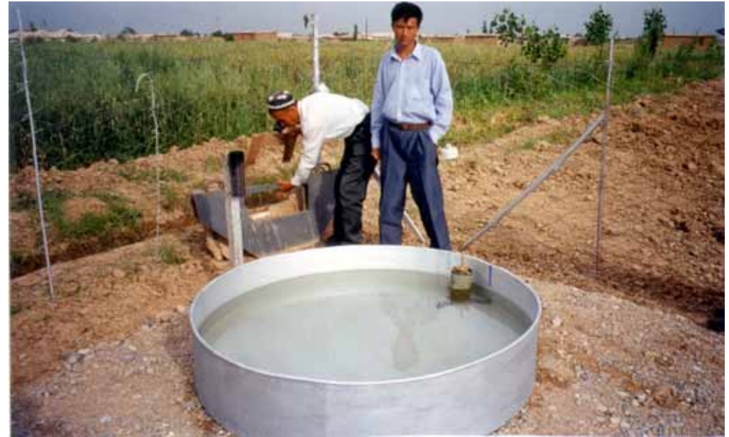
Evaporimeter, rain gauge and portable weir introduced by WUFMAS as the basis for on-farm irrigation scheduling
