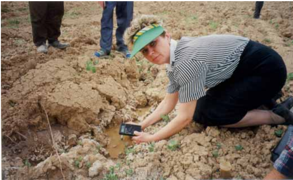
Local meter reveals highly saline ground water at soil surface - abandoned demo field, Farm 22, Surkhandariya
